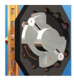
During the turn movement, the safety pins [1] are moved along the swivel clutch [3] into further recesses [2] where they again audibly engage.
