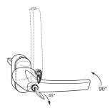
The lockable Roto Tilt-First handle (tilt before turn) locks the window sash in the tilt mode, with the handle in the horizontal position. The lockable handle prevents the possibility of changing from tilting to turning in order to fully open the window. This is only possible after unlocking.
